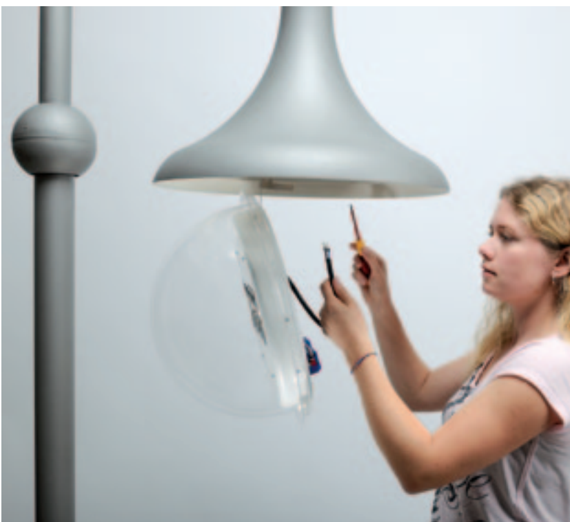
The LED module is fastened to the housing via a retaining wire. This means both hands are free for the connection.
