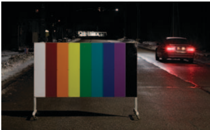
Streetlight 10 – pleasant, neutral white light for good colour rendering. Ra>70
