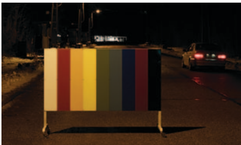
HST – road and vicinity have a yellow tinge. Colour rendering is poor. Ra<40
