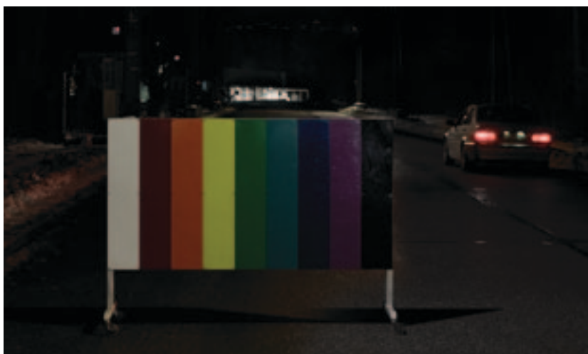
HME – road and vicinity have a blue-green tinge. Colour rendering is limited. Ra 45–60
